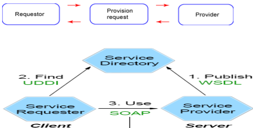
Figure 1: Web services Architecture
